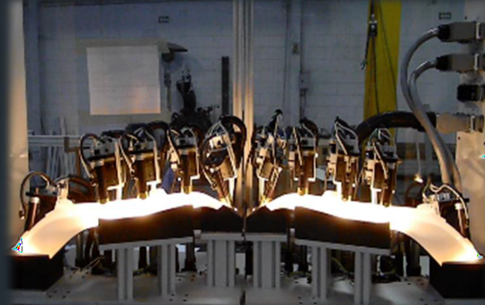
Infra Stake Welding
